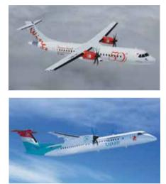
original Dash 8-100 (Series 100) entered service in 1984 and has a maximum capacity of 39 seats. The Series 200 has the same capacity but offers more powerful engines, the Series 300 is a stretched 50seat version and the Series 400 is a further stretch originally seating a maximum of 78 passengers, which has subsequently been pushed to 80, with a 90-seat configuration in development.
