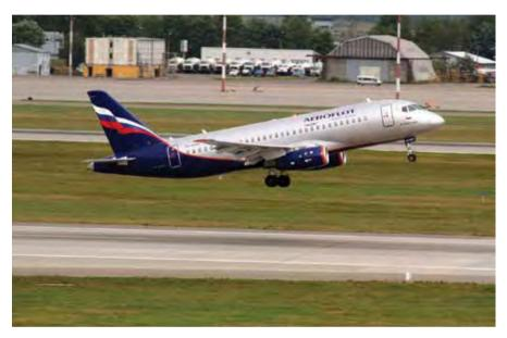
aunched in 2000, the Sukhoi Superjet 100 (SSJ100) is a product of a joint venture between the Russian aircraft manufacturer Sukhoi and the Italian aerospace company Leonardo. It is a new-technology, fly-by-wire regional aircraft powered by two PowerJet SaM146 engines, jointly designed and produced by Snecma Moteurs and NPO Saturn. The aircraft has the highest-ever proportion of western components in a Russian aircraft.
