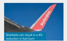
are large wingtip devices that the manufacturer says can result in a 4% reduction in fuel burn over longer sectors.
