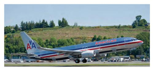
upgraded CFM56-7BE engine enhancement programme to coincide with airframe improvements. Boeing said at the time that the combination reduced fuel consumption by 2%. The
