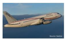
Holding and Alenia Aermacchi, a division of Italian aerospace conglomerate Leonardo (formerly known as Finmeccanica). The current-production models are the 100-seater SSJ100 in Basic version with a range of 3048 kmand a long range (LR) version of 4578 km range.
